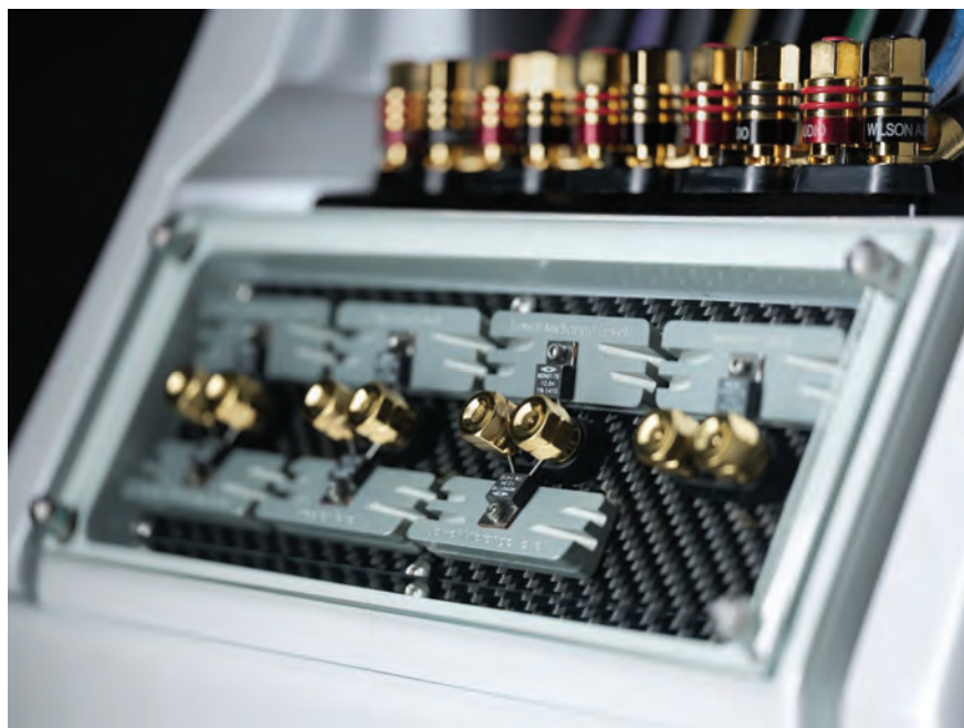
The fusible driver protection resistors and tonal balance adjustment panel
